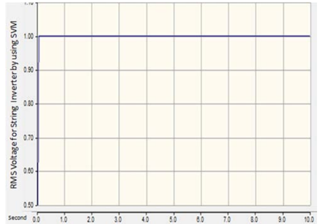
Figure 21. RMS-output of string inverter using SVM.
