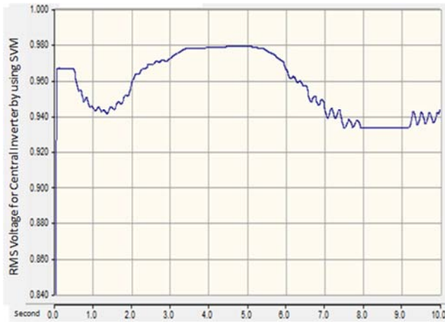
Figure 18. RMS-output voltage of central inverter Using SVM.
