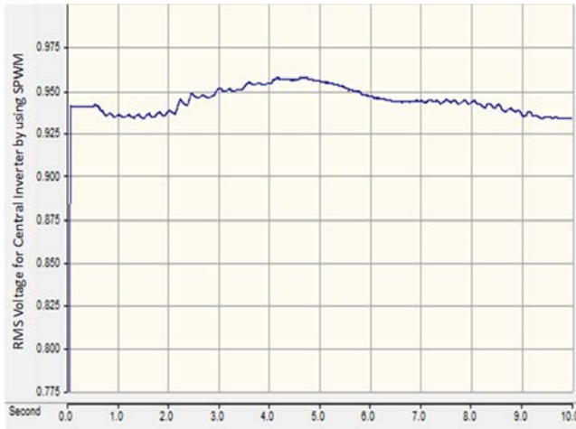
Figure 12. RMS-output voltage of central inverter using SPWM.
