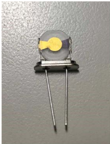
Figure 3. A photograph of a QCM sensor.
