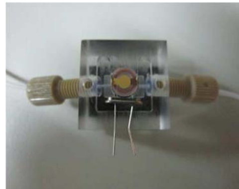
Figure 5. A QCM sensor was mounted by concentric rubber seals into a flow cell.
