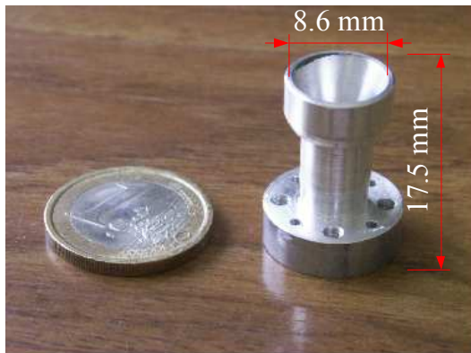
Fig. 10.a. Prolate horn antenna
